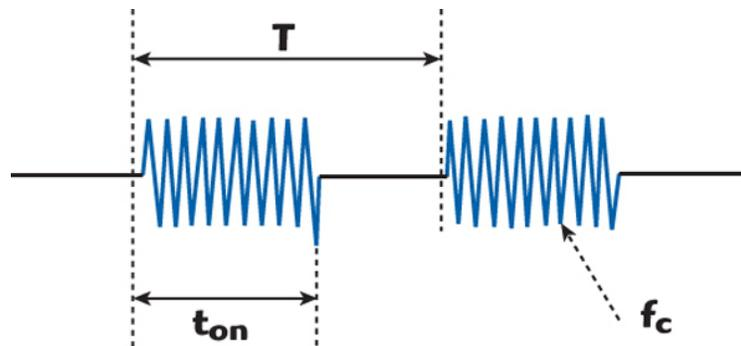
**Figure 1—Example of a rectangular wave modulated at a carrier frequency  $f_c$ . For the Sensormatics anti-theft device waveform,  $f_c = 58$  kHz,  $t_{on} = 1.6$  ms, and  $T = 16.6$  ms.**
