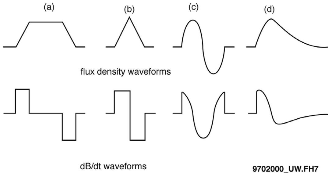
**Figure 2—“Broadband” waveforms of flux density,  $B(t)$  (upper), and its time-derivative  $dB/dt$ , that have been used as MRI switched gradient fields. The repetition period,  $T$ , in MRI scans could be greater than the “on-time” of the waveform. Note that examples (a), (b), and (d) of the flux density waveforms,  $B(t)$ , are monophasic, while all the  $dB/dt$  waveforms are biphasic and charge-balanced (zero net charge). (From Reilly, 1998, Fig. 9.14).**
